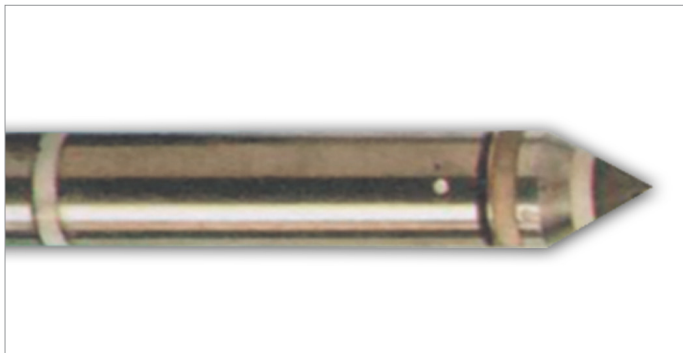
Porous elements in the shoulder of the cone
