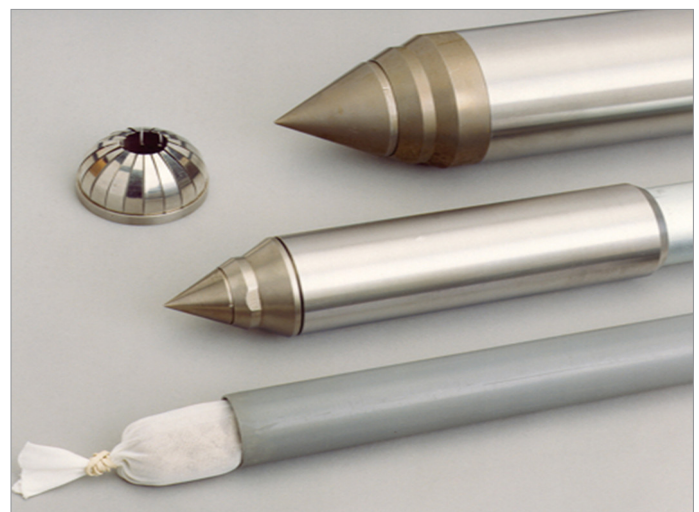
Soil sampling during CPT tests for laboratory testing
